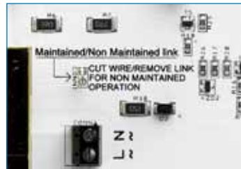
Configurable as Maintained or Non-Maintained operation
